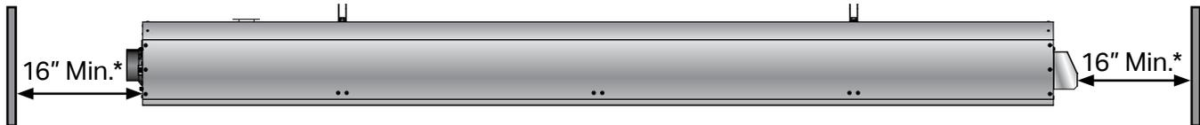
\* Minimum end clearances are 16". However, these distances may be greater when taking into account accessibility of the controls compartment, heat tolerance of adjacent materials such as plastic, and air flow requirements.
