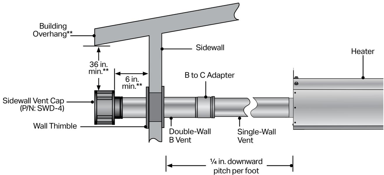
\*\*Vent must extend beyond any combustible overhang if the vent is less than 36 in. below the combustible overhang.
