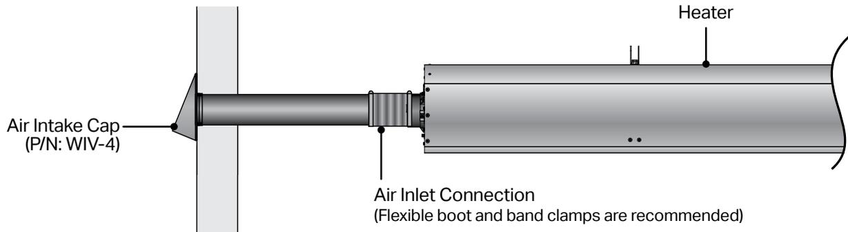
Figure 3.12 • Vertical Combustion Air Intake - Side View
