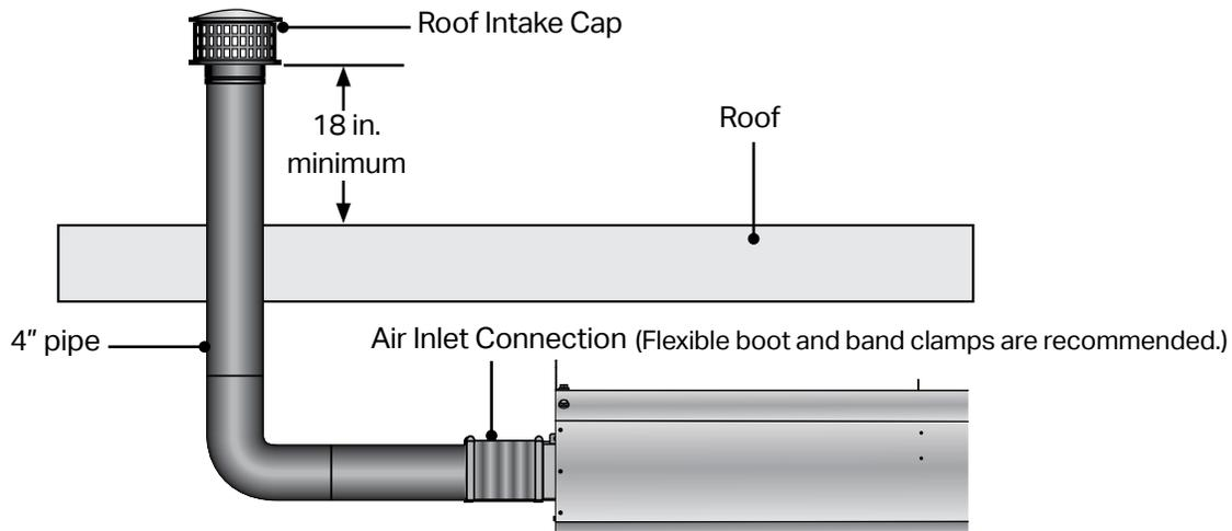
Figure 3.13 • Outside Combustion Air Sidewall Intake - Side View
