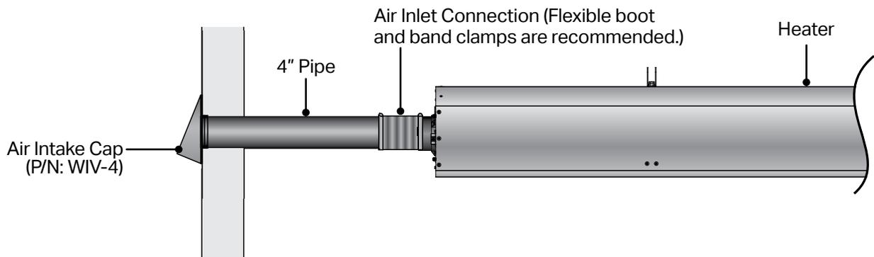
Figure 3.14 • Vertical Outside Air Supply for Common Intake - Side View
