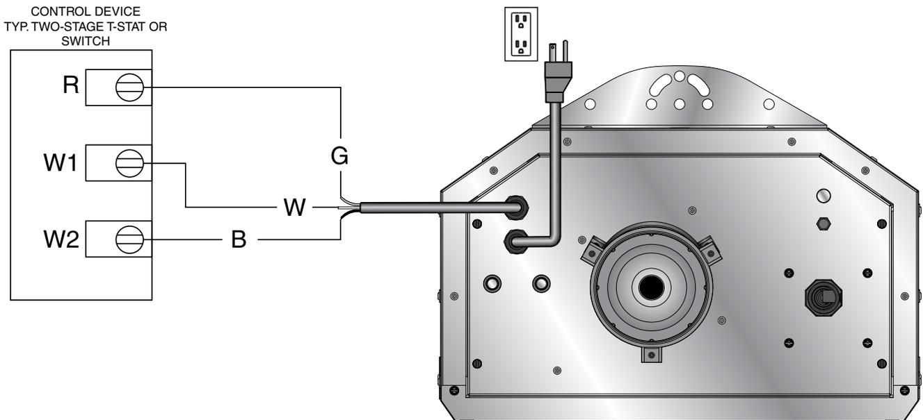
**Figure 3.19 • Field Wiring Diagram - Controlling Multiple Heaters with a Single Control Device Utilizing Optional External Relay Kit (P/N: ERK)**
