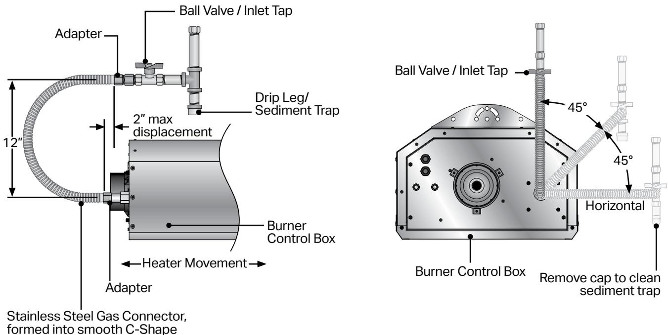
In Canada, infrared heater shall only be connected with a Type I hose connector that is (a) certified as being in compliance with the *Standard for Elastomeric Composite Hose and Hose Couplings for Conducting Propane and Natural Gas, CAN/CGA 8.1*; and (b) of a length of  $36 \pm 6$  in ( $90 \pm 15$  cm).
