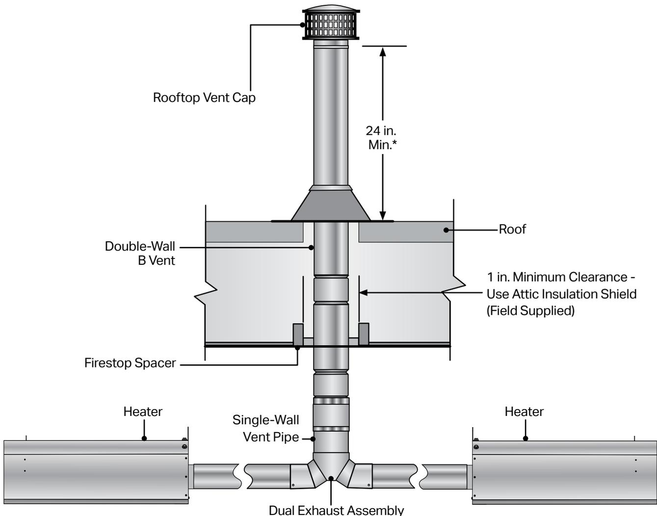
\*Consult the NFPA ANSI Z223.1 Gas Vent Termination criteria if roof pitch exceeds 9:12.
