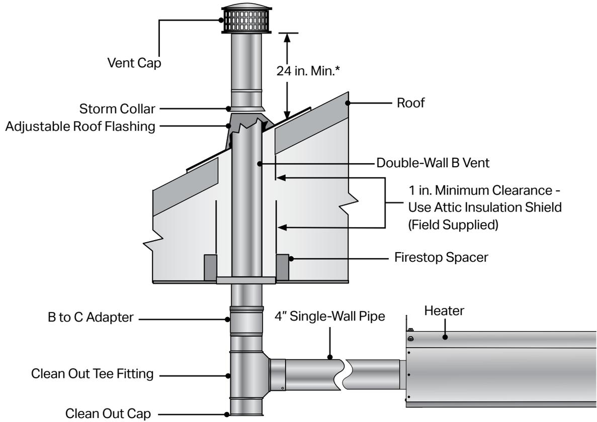
\*Consult the NFPA ANSI Z223.1 Gas Vent Termination criteria if roof pitch exceeds 9:12.
