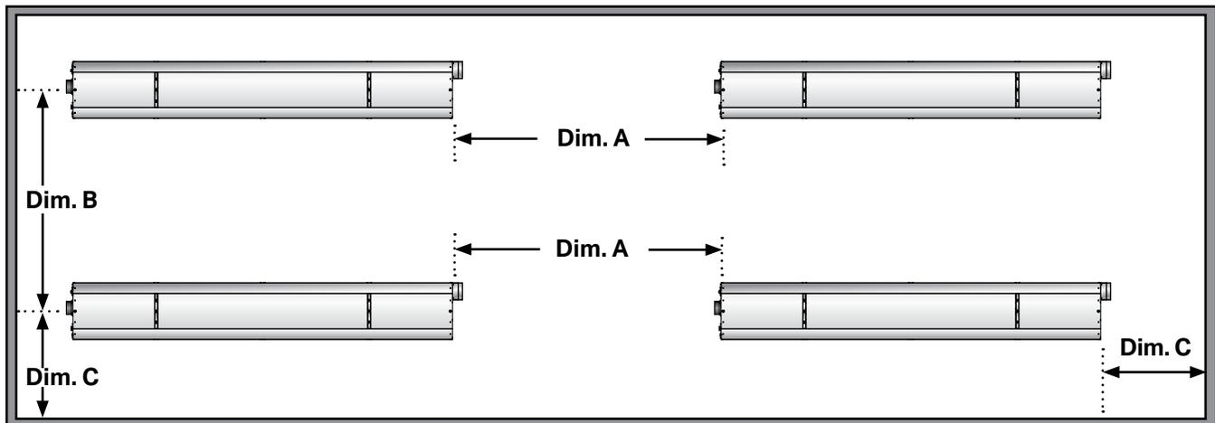
**NOTE:** Dimensions A, B, & C are based upon heaters hung at the factory recommended mounting height.
