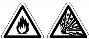
Testing for gas leaks with an open flame or other sources of ignition may lead to a fire or explosion and cause serious injury, or death. Test in accordance with NFPA or local codes.
